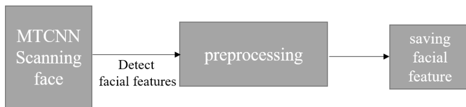
Figure 1. Facial Recognition Preprocessing Flowchart
