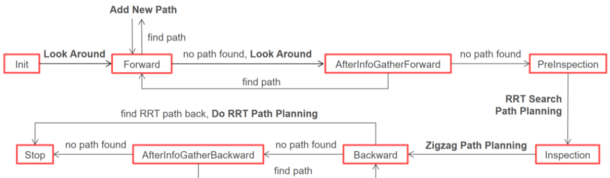
Figure 5. Path planner finite state transition logistic overview. The plain normal font means the
